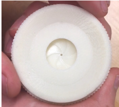
Figure 4: Left: The first complete 3D printed assembly. The parts had a very tight fit at first and we had to sand them down to achieve a smooth rotation.
