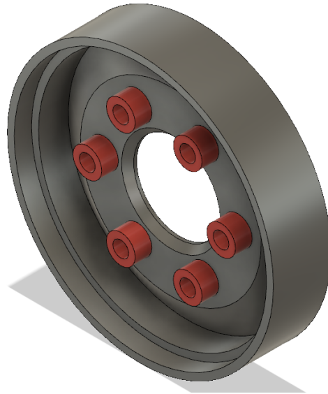
Figure 1: This is the design of the front of the yo-yo used for the first prototype. The bosses shown are used to hold the leaves in the iris mechanism. The hole in the center is where the lens bubbles out. This design would have caused difficulty in assembly, though, because the lens dome would have to be a non-circular shape to fit between the bosses; that reason also made it hard from a manufacturing standpoint.
